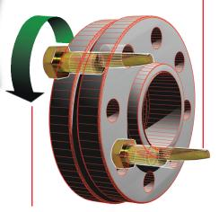
**Step 2:** Place second bolt into mis-aligned holes and turn bolt to align both flange faces
